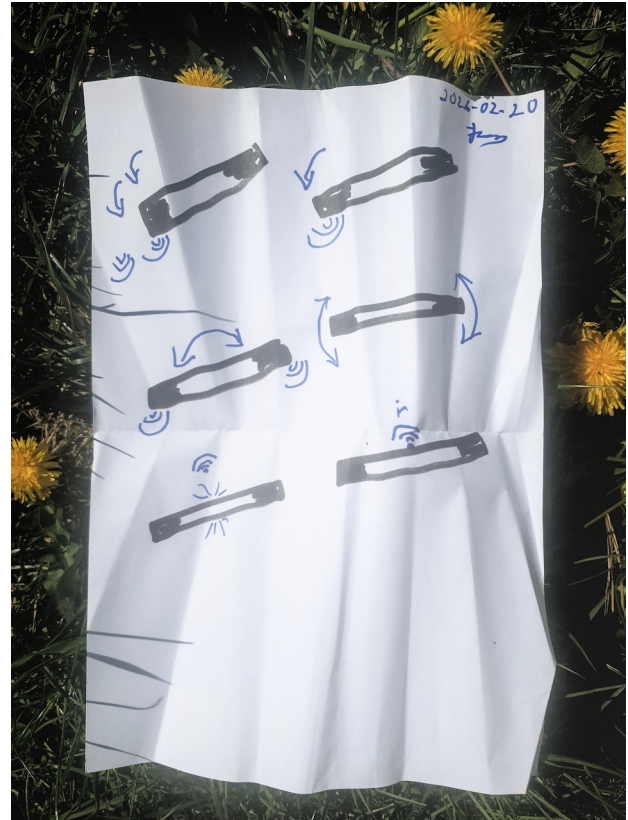
Figure 4: Counting wand sketch, with ideas for interaction: Counting by tapping, changing consumption type by double-tapping, tapping at both ends or tilting the wand to the sides, and reading the counted data via wifi or infrared transmitter.
